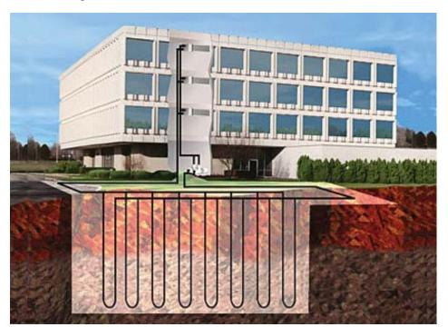
An illustration of a geothermal system that shows how underground pipes circulate water that is then used for heating and cooling.
